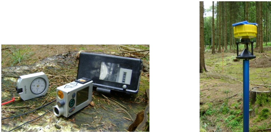
Figure 2.3 Equipment: (Left) from left to right Suunto compass, Vertex telemeter, and Walktux distance measurer. (Right) Transponder on plot centre staff.
